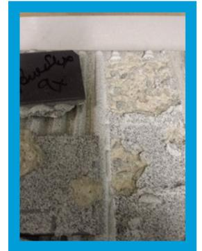
Powerflex Grey is ideal for adhering to early age concrete. Screeds should be cured for 7 days, then allowed to air dry for a further 14 days according to Australian Standards AS3958 part 1 2007. Morgan's quality assurance program reflects the continual testing of our products by our chemist. We test to Australian and International Standards to ensure our products meet all the requirements for both performance and health.
